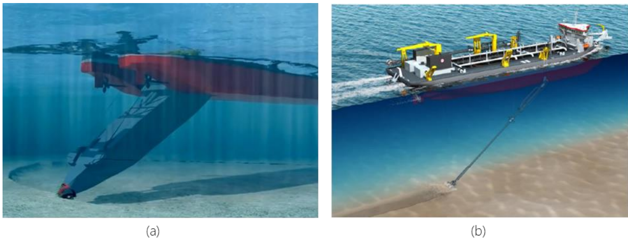
Figure 3-8 - (a) Cutter suction dredger (b) Trailing suction hopper dredger
