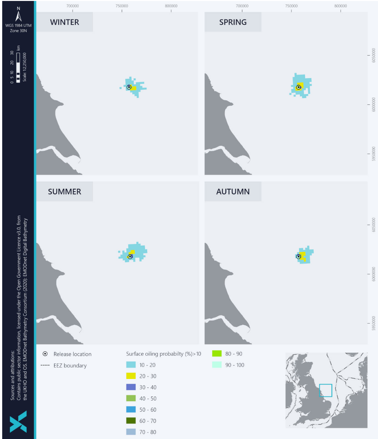
Figure 10-5 - Scenario 1: Loss of entire rig diesel inventory instantaneously at the Endurance Store – Probability of surface oiling (above 0.3 \mu m) above 10%
